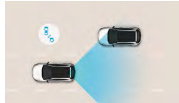
Blind Spot Collision Warning (BCW): Radars detect traffic in the vehicle blind spot, warning drivers with an audible alarm when the indicator is used so you can be aware of the traffic around you even when you can't see it. Available on Premium and Ultimate trims only.
