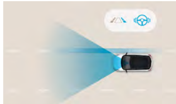
Lane Keeping Assist (LKA): The Lane Keeping Assist (LKA) uses the front multi-function camera to monitor the lines of the road. In case of an unintended lane departure, it warns you and can apply counter steering torque to guide the car back to the lane.
