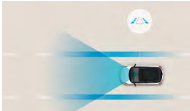
Lane Follow Assist (LFA): Smart sensors and the forward-facing camera detect when the car drifts from the centre of the lane, applying steering torque to maintain road positioning for safety. The car also estimates the trajectory of the vehicle ahead and adjusts its position accordingly. Available on Premium and Ultimate trims only.
