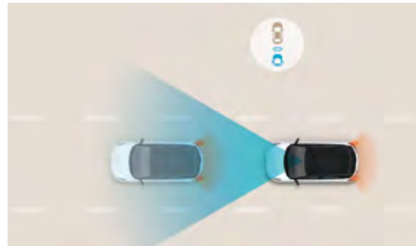
Front Collision Avoidance (FCA): The front view camera and radar sensors warn drivers of imminent collisions with vehicles and objects, applying the brakes when necessary to avoid collisions.
