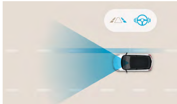
Highway Driving Assist (HDA): For additional safety, Highway Driving Assist keeps your vehicle at your pre-set speed and maintains road position in your lane. HDA monitors the distance to the vehicles ahead, reducing speed automatically when the gap closes. When the safe distance is restored, HDA resumes the pre-set cruising speed.
