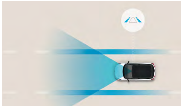
Lane Follow Assist (LFA): LFA helps prevent accidental lane departure and keeps your vehicle safely centred within the lane. Using a forward camera to recognise the intended lane, LFA will automatically provide corrective steering input to help maintain the centre path. This not only detects road lines but also the road edge.
