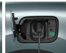
Charging Mode in Progress (Flashing green LED)
