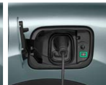
Charge Complete Mode (Constant green LED)
