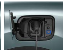
Deferred Charge Mode (Flashing blue LED)
